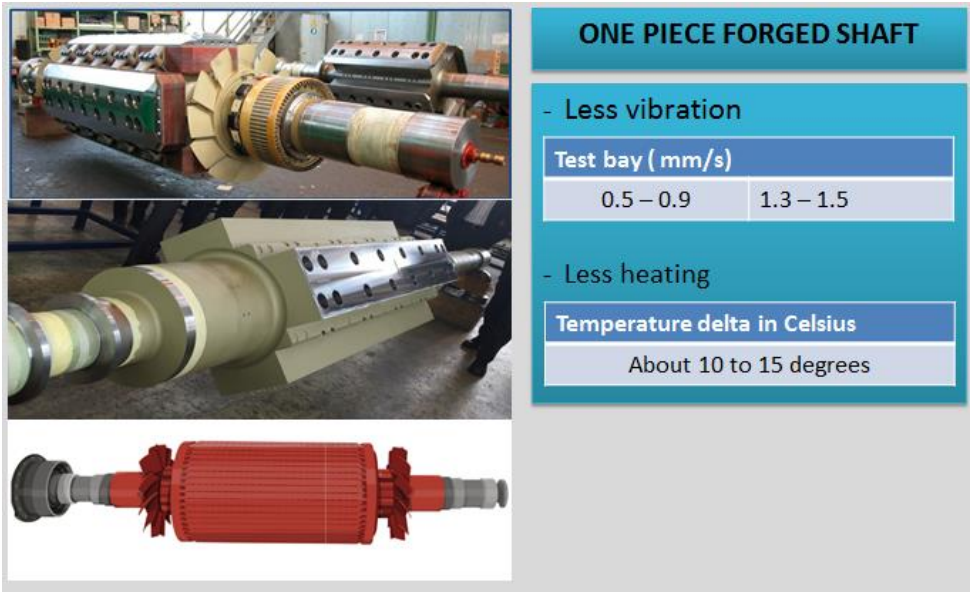
Figure 6: Rotor construction
