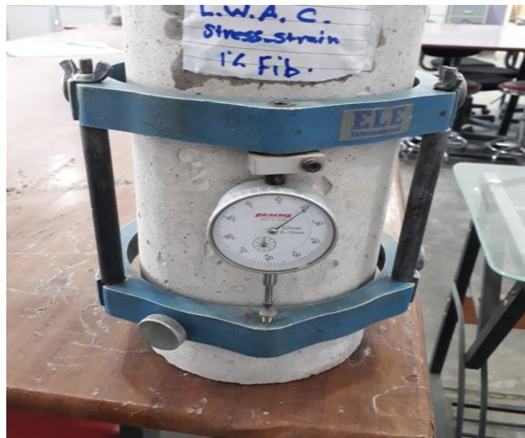
Fig.3 : Lightweight Aggregate Concrete Cylinder Before Testing To Stress-Strain Diagram.
