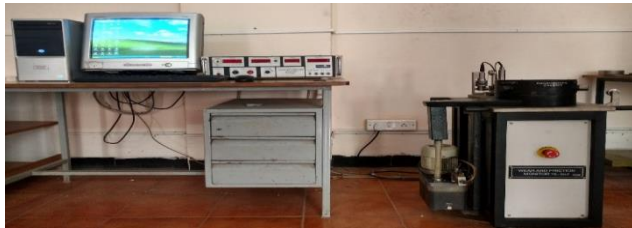
Fig. 2: Pin-on-disc Setup and Wear Monitor
