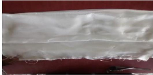
**Fig: 1 Bidirectional roving E-glass fiber mats**
