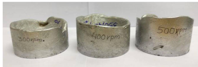
Fig 3.2. Cast of 6mm thickness of Al 5% Si with 1% Zirconia reinforcement
