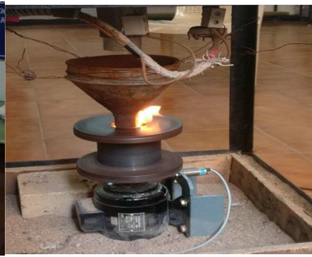
Fig 2. Vertical Centrifugal setup
