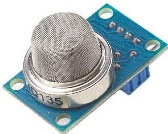
FIG 4: MQ-135 Alcohol Sensor
