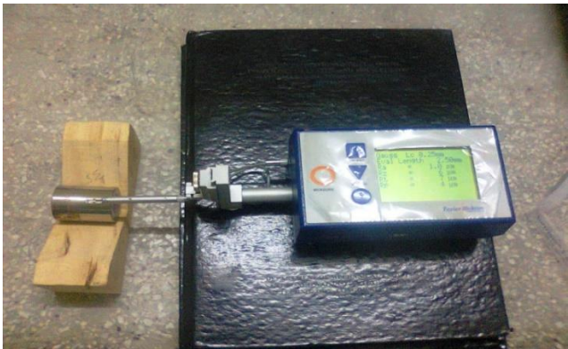
Figure 5: Surtronic 25 (Metrology lab, Mechanical department, SLIET)
