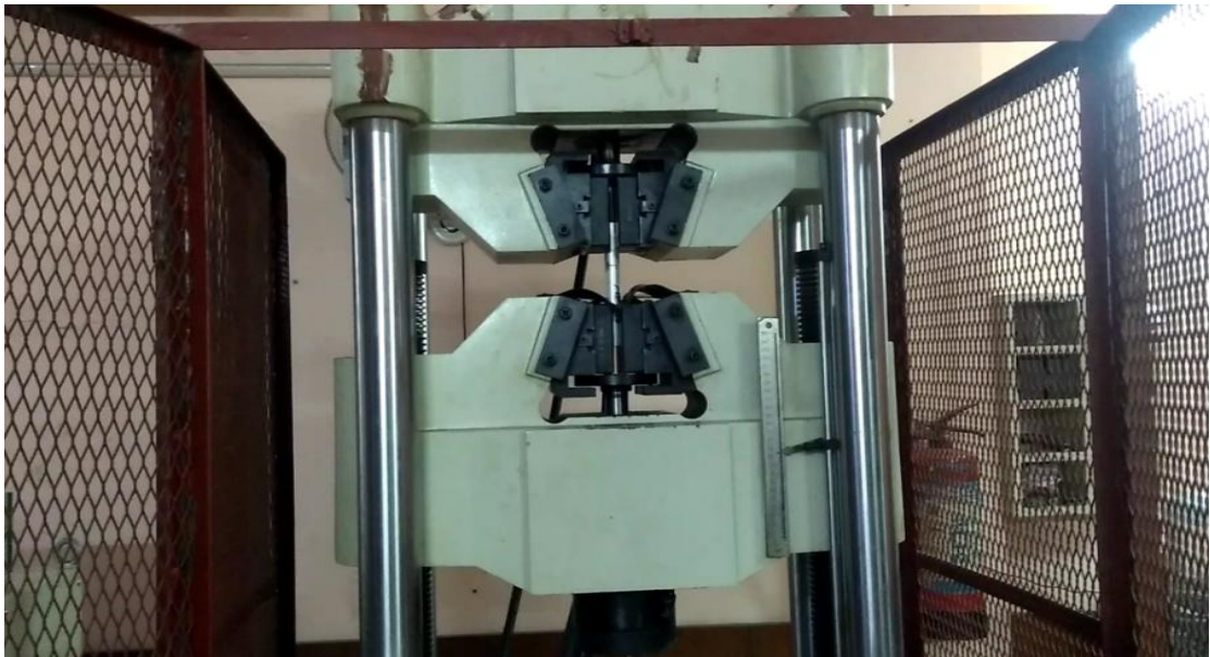
Fig.6. Setup of tensile testing
