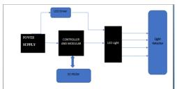
As block digram shows transmitter side, unique identification is to be assign by the microcontroller and control headlight through LED driver and light shows its unique identification.
