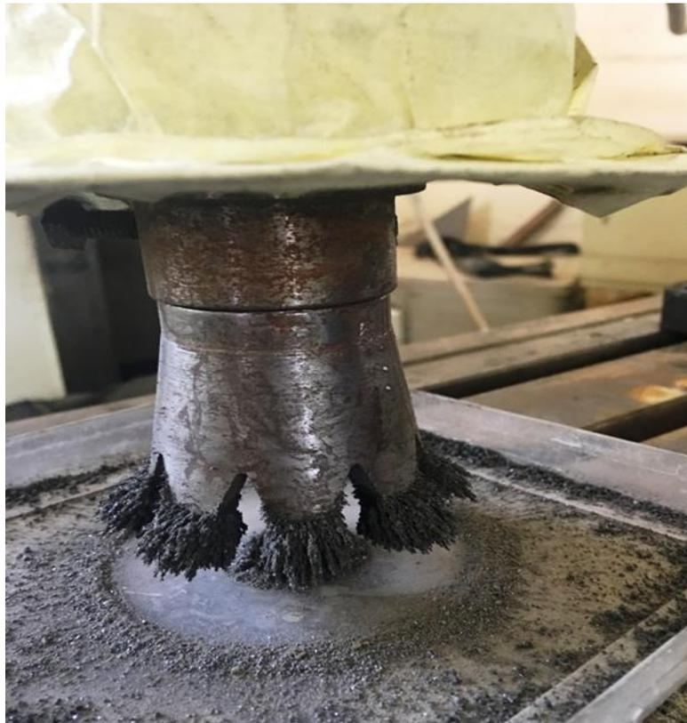
Figure (4) machine of MAF process
